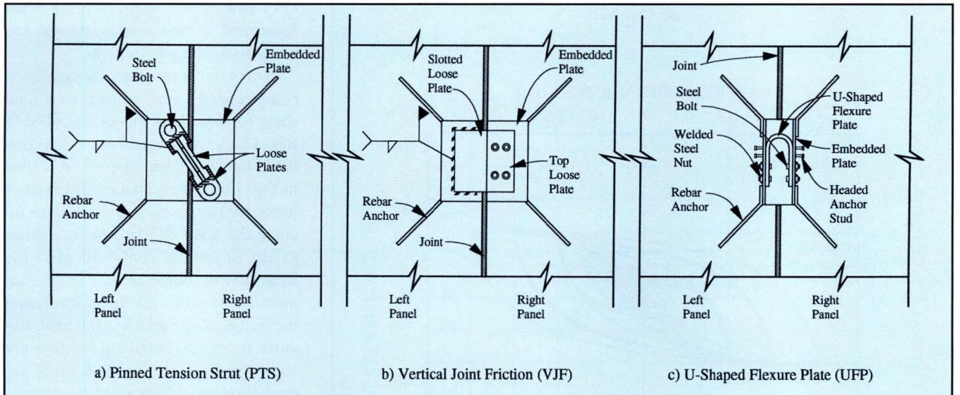
Fig. 8. Bolted ductile connections tested at NIST.
