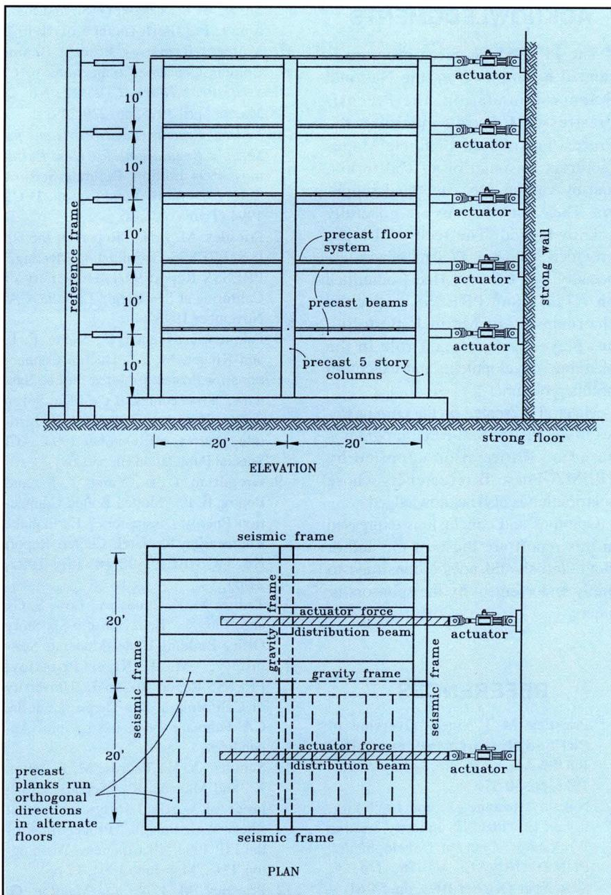
Fig. 20. Eight-tenths full-size precast frame super-assembly.
