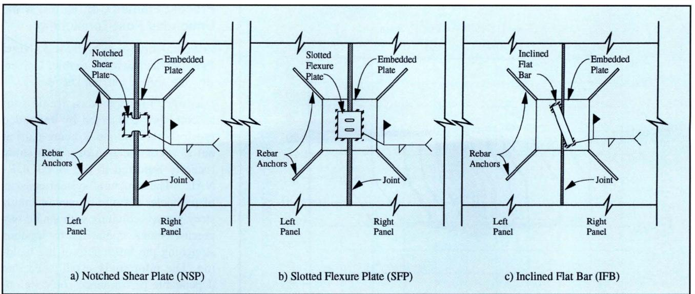
Fig. 7. Welded loose plate connections tested at NIST.
