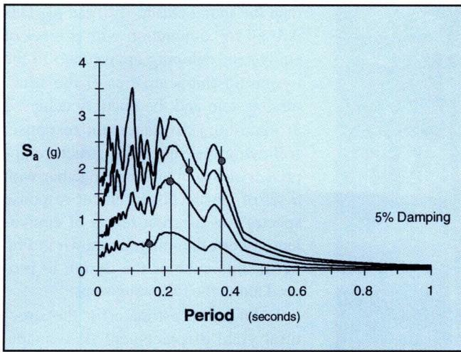
(a) Spectral response curves for Test Runs 1-4
