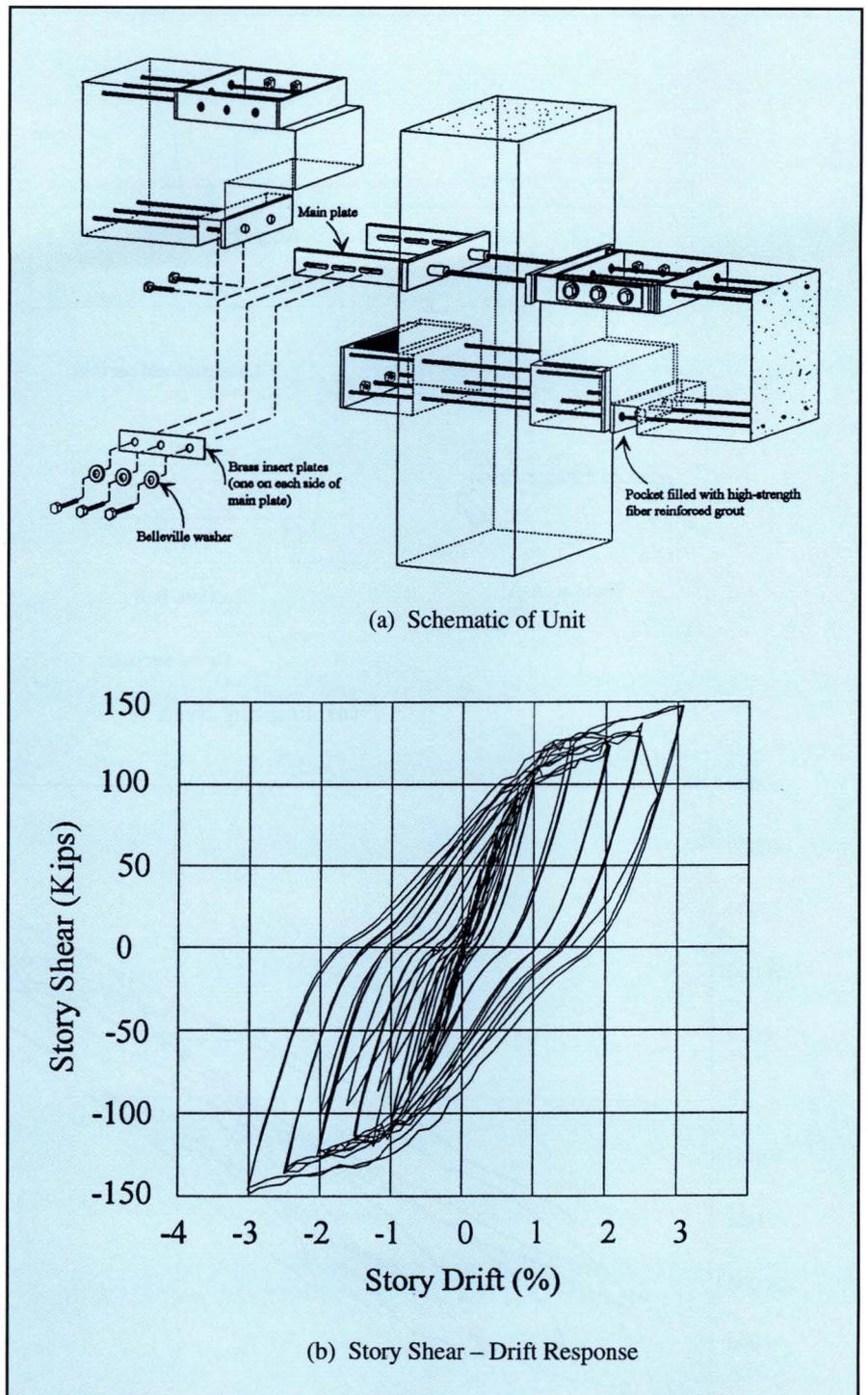
Fig. 5. Unit UT-FR added-damping subassembly (University of Texas at Austin).
