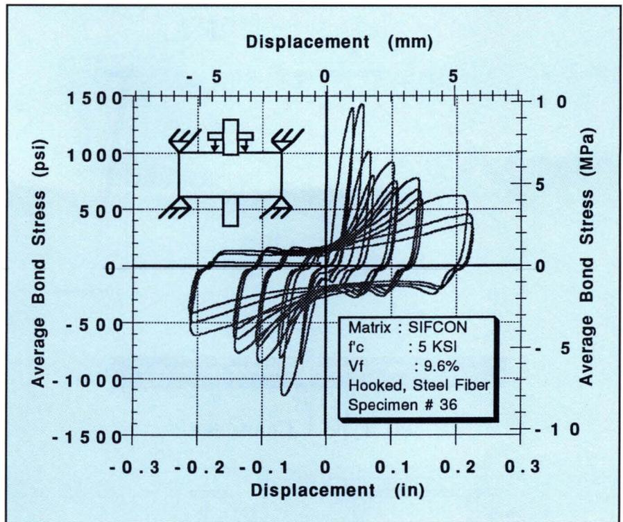
Fig. 14. Bond stress-slip response for a reinforcing bar in SIFCON concrete (University of Michigan).
