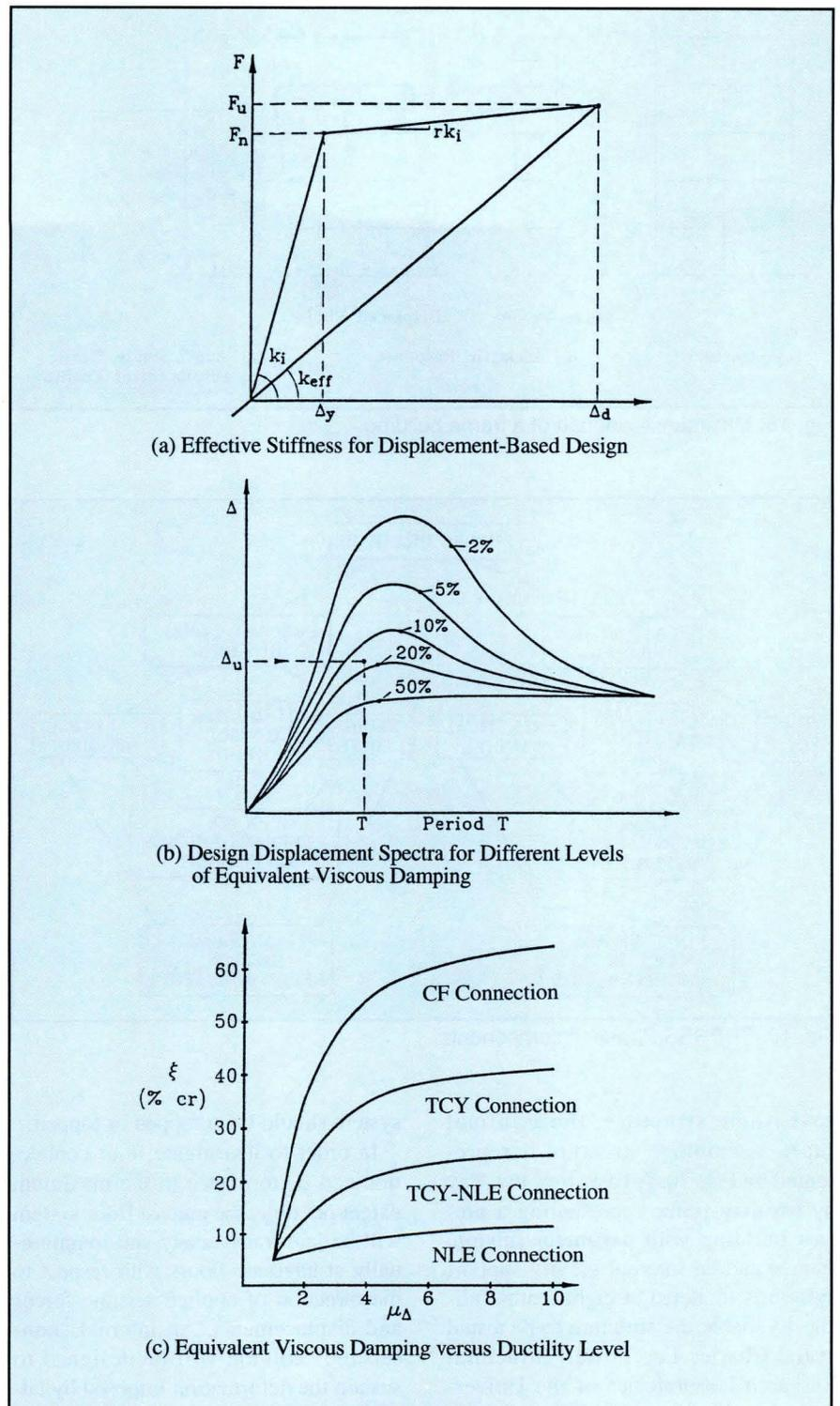
Fig. 17. Elements of displacement-based design procedure.
